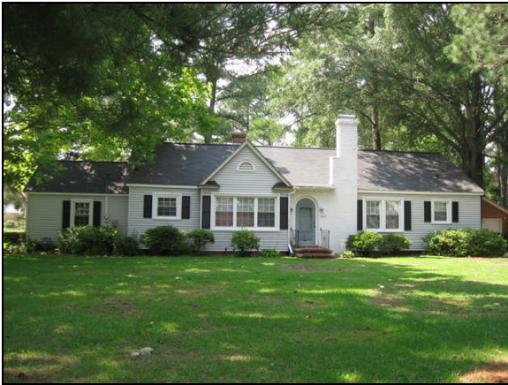
1302 Respass Street. This frame house displays elements of the Period Cottage style such as arched entry, front facing gable and façade chimney.
